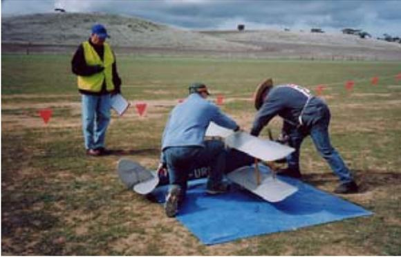
Ian Crowhurst of South Australia starts his DH 60G III (Moth/Tiger) in the start box. Model is 1/4 scale and powered by an OS 120 mounted inverted.
