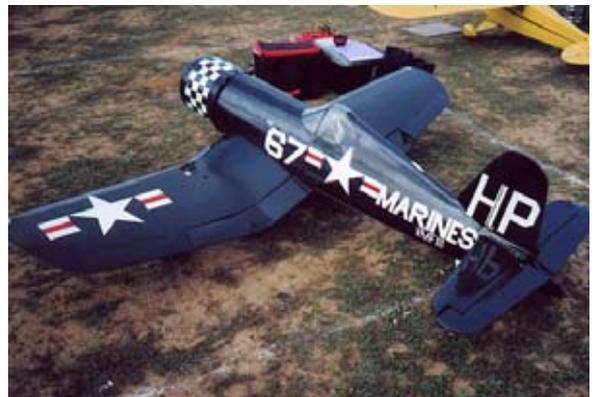
Vought Corsair by Trevor Gale of South Australia. Model is 2.36m span and weighs 19.5kg. Power is a Zenoah 74 twin.
