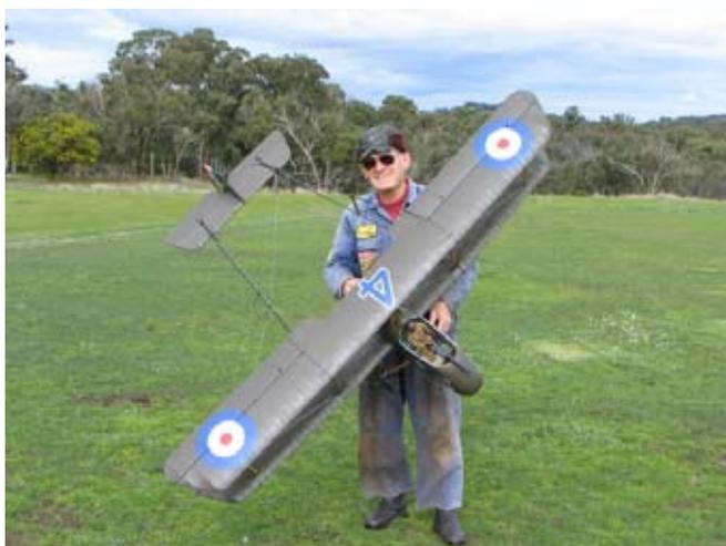
combination were overcome. The long span wings, and lighter weight, as compared with my old S.E.5a, provide an excellent rate of climb, and level flight could be maintained at about half throttle. In fact the F.E.8 is a bit fast at full throttle and a 70 or 80 size four
