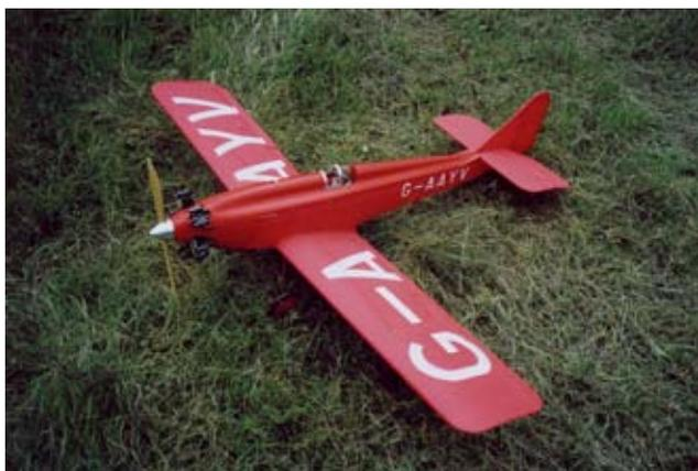
The Avro had a radial engine and David built this up from a Williams Bros. Moulded cylinders. The model is powered by an inverted Taipan 2.5cc diesel and is to one eighth scale for a weight of just over two pounds or 1kg. With a low wing and not much dihedral it will also be a challenge to trim!
