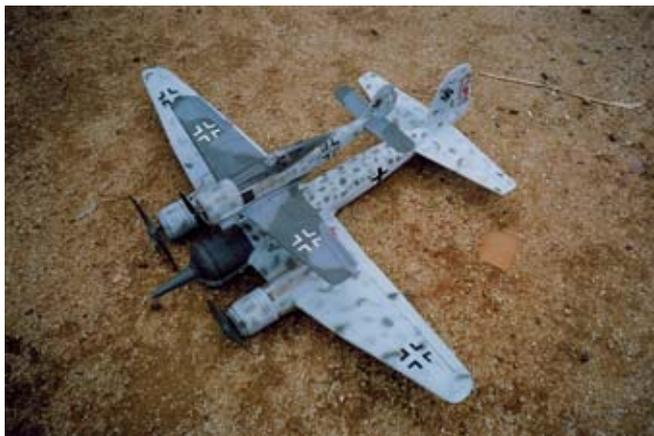
David's model has three electric motors and two batteries. The FW190 has one KP-01 and the twin has two KP-02. A timer mechanism operates about 20—25 seconds after launch and, in theory, the two modes separate and fly away.
