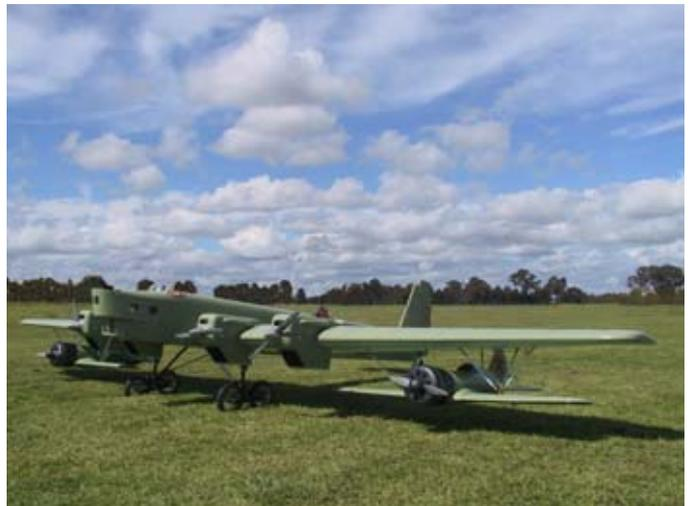
The Tupolev TB-3 powered by four 0.46 engines and with the electric Polikarpov I-16's under the wings.
