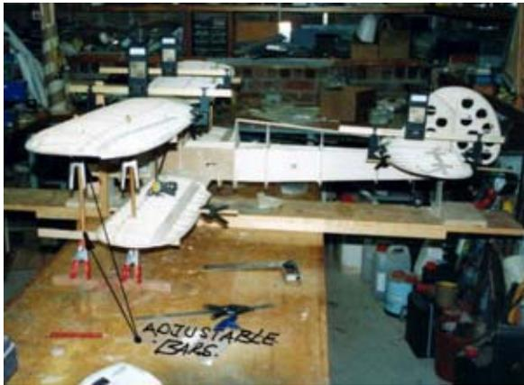
The aircraft jugged up for correct setting of wing and tailplane incidence. Barrie has invested heavily in Robart incidence meters.
