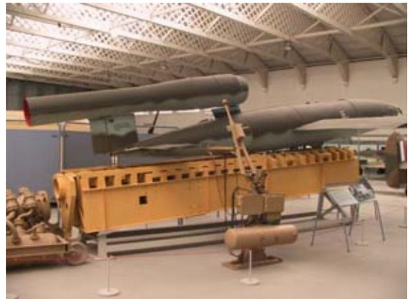
German V1 Flying Bomb on a section of launching rail. The V1 was powered by a pulse jet.
