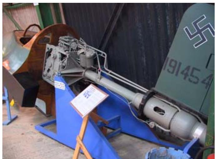
A mock-up of the Messerschmitt Me 163 showing the Walter rocket motor which produced 750kg of thrust for 71/2 minutes, propelling the 4300kg aircraft to nearly 1000kph.
