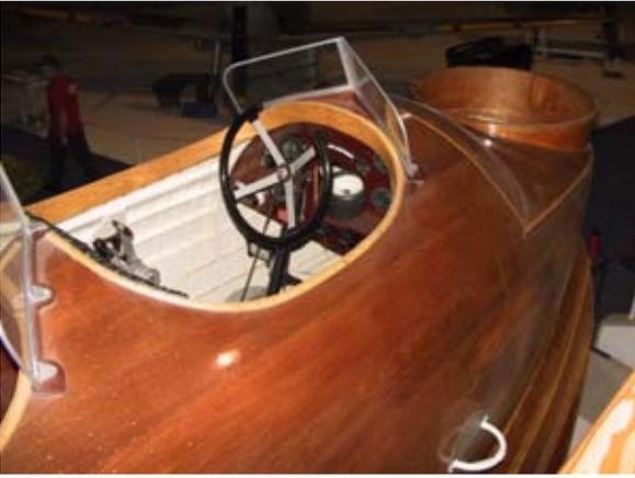
Beautifully restored woodwork on this Supermarine Southampton flying boat from the 1920's. More than 75,000 small screws were used in the restoration.
