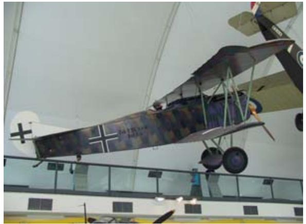
The Fokker D.VII designed by Reinhold Platz was the premier German fighter of WWI. It first saw service in 1918 and was superior to the French SPAD and the British S.E.5 and Camel.
