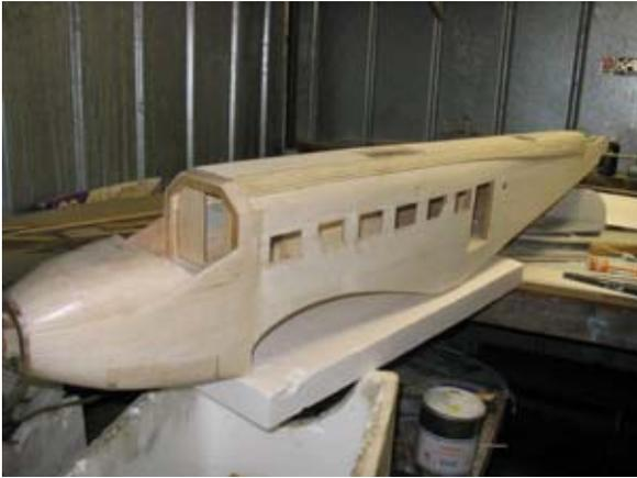
I started building last July and progress was rapid until I was confronted with the corrugations on the tail feathers and the fuselage. Having spent some time trying to work out the scale size of each corrugation I found that there were three different sizes. In an effort to keep the weight down I decided to make the corrugations out of strips of balsa.
