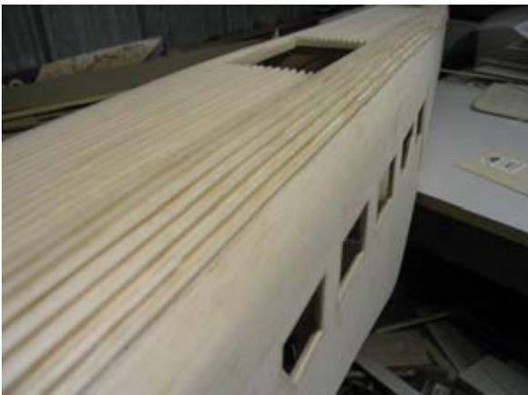
Once an area is corrugated it must be sanded down to a uniform height. I used a piece of brass tube of the desired diameter placed between the corrugations to sand down to. Next I made up a sanding block, a short length of 3/8" square hard wood with sandpaper
