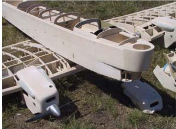
The TB-3 mother ship is conventional balsa/ply construction and will be covered with Solartex.
