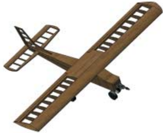
Figure 7: Trainer model used in flight tests (wingspan = 1.6 m).
